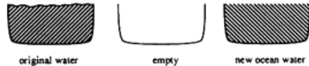
Option 1. emptying + refilling (Reballasting)
